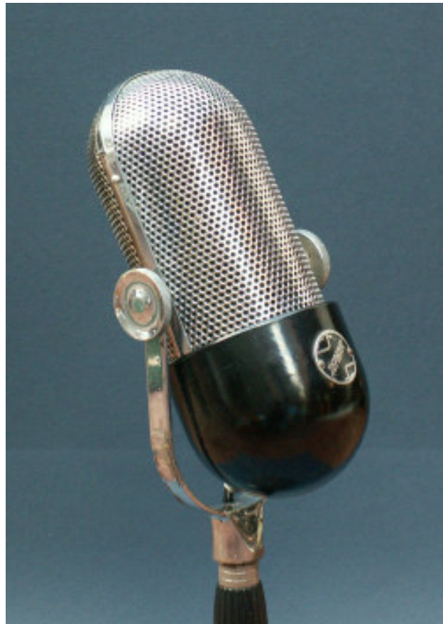
Zephyr is a '40 series'. Circa 1952 Fig 8 ribbon. Made in Australia 'A high fidelity studio microphone with real artist appeal" and at a reasonable price. Designed for musical and high quality speech reproduction.' One of Zephyrs 'Top Three' microphones.
