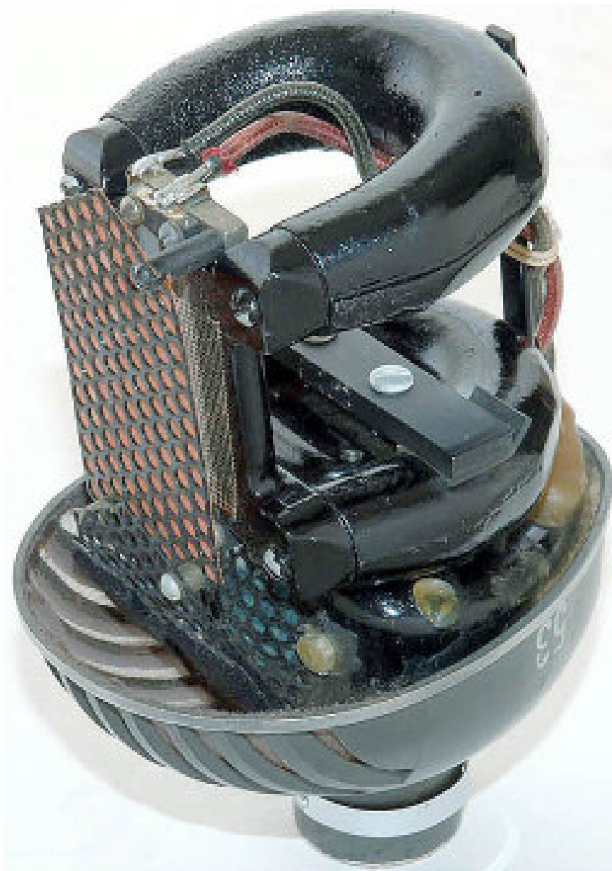
The Western Electric 639A. 1939. Altec later purchased Western Electric. Three switch selectable patterns are non-directional, figure eight, and cardioid. Combines a dynamic moving coil pressure element (non-directional) and a ribbon velocity element (figure 8). The later 639B has 6 patterns.
