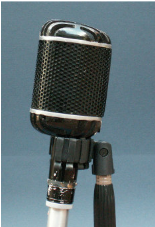
STC 4033A STC's version of the Western Electric 639A. Three switch selectable patterns are non-directional, figure eight, and cardioid. Combines a dynamic moving coil pressure element (non-directional) and a ribbon velocity element (figure 8).
