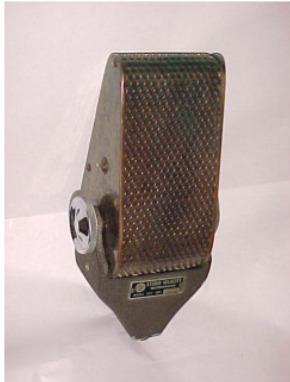
Steanes R47 Fig 8 ribbon. Made in Australia.
