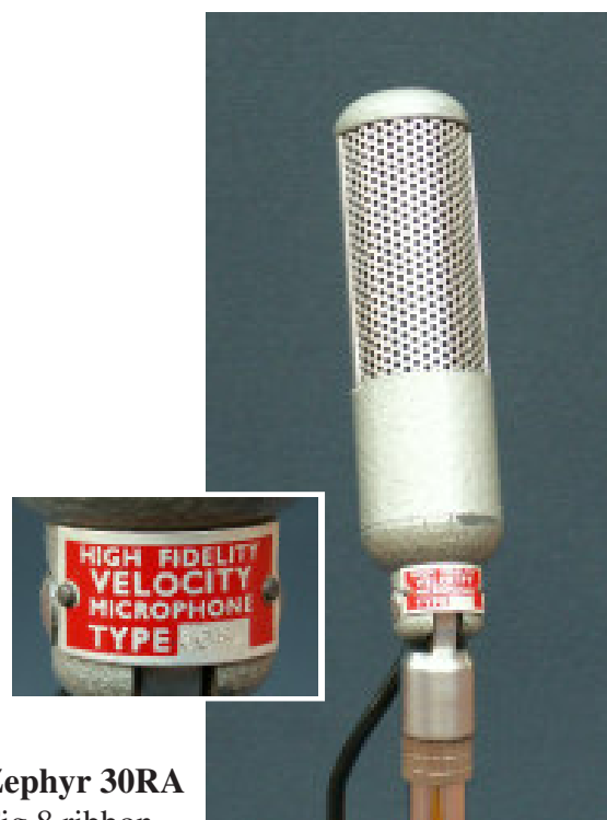
Zephyr is a '40 series'. Circa 1952 Fig 8 ribbon. Made in Australia 'A high fidelity studio microphone with real artist appeal" and at a reasonable price. Designed for musical and high quality speech reproduction.' One of Zephyrs 'Top Three' microphones.
