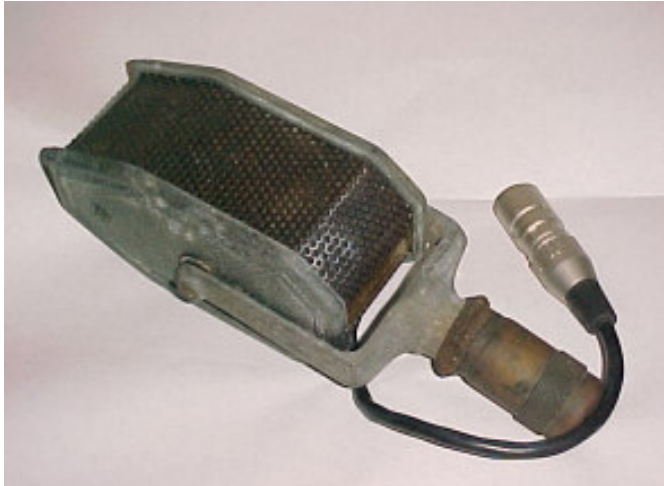
Amperite RBM 1930s Fig 8 ribbon. Made in Chicago.
