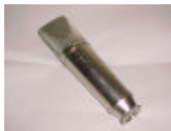
Rode NT1 (Neumann clone) Cardioid condenser. Made in Australia.
