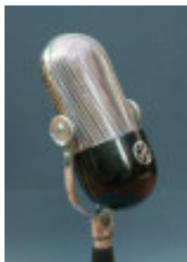
Zephyr is a '40 series'. Circa 1952 Fig 8 ribbon. Made in Australia
