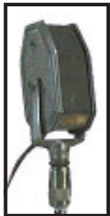
Amperite RBM 1930s Fig 8 ribbon. Made in Chicago.
